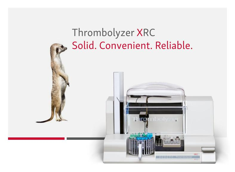
The Thrombolyzer XRC is a fully-automated in vitro coagulation analyzer which delivers high quality results and meets the demands of mid-volume labs with easy, intuitive usage.
